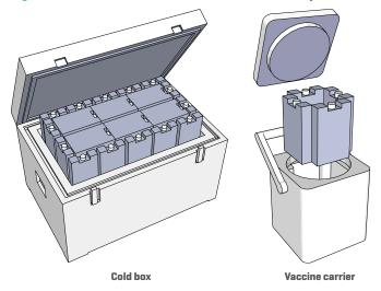
As part of the WHO prequalification process, containers are laboratory tested under controlled conditions. These tests assess whether the product is robust enough to withstand longterm use and establish its cold life, cool life, and warm life.
